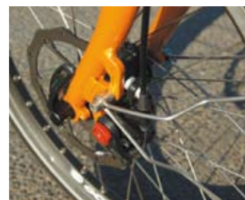
ABOVE: Tidy work on the mudguard stays to accommodate the disk brake.
